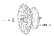
2. Insert the motor into the frame.
